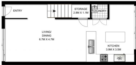
GROUND FLOOR GROUND FLOOR
